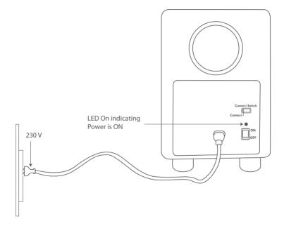
Note: Check LED is "ON" when connected to Power source
